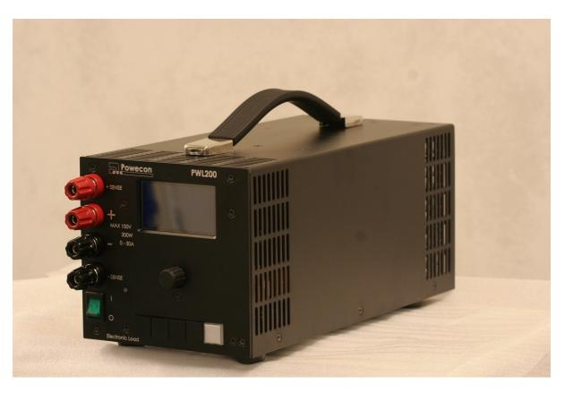
PWL electronic loads are reliable and usable equipment intended for professional power electronics testing. They are designed to fulfil reliability and life time demands needed in long term reliability and production testing in electronics industry.
